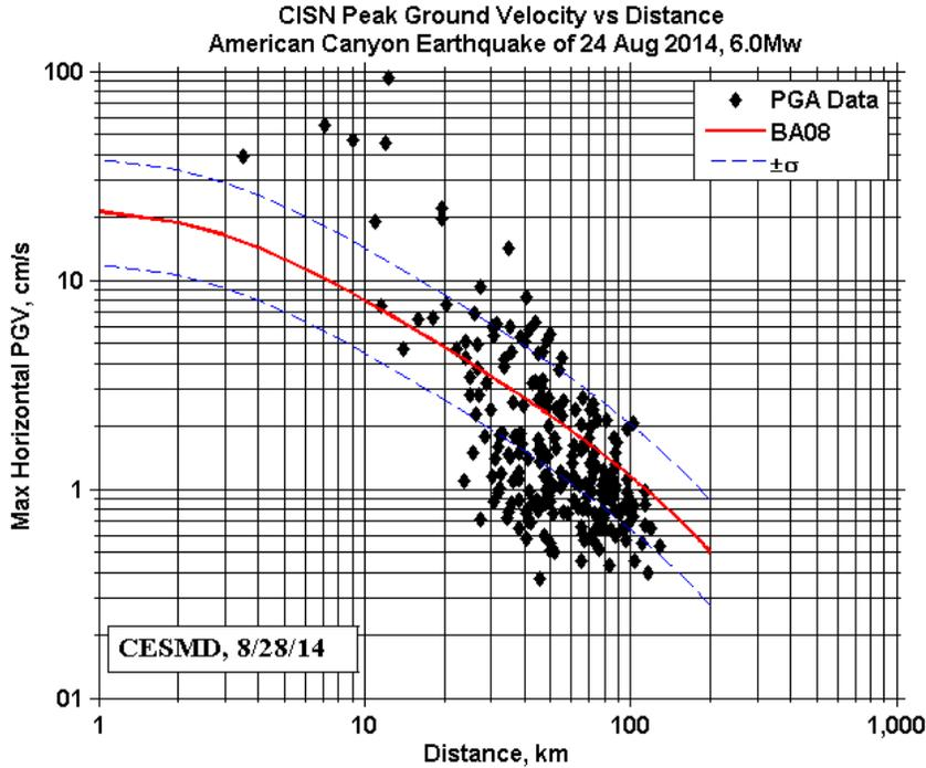
Figure 2. Plot of PGV vs. epicentral distance compared with the NGA ground motion prediction equation of Boore and Atkinson (2008).
