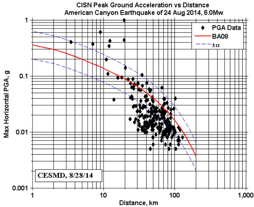
Figure 1. Plot of observed PGA vs. epicentral distance compared with the NGA ground motion prediction equation of Boore and Atkinson (2008).
